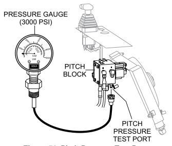
**Figure 51. Pitch Pressure Test Port**
